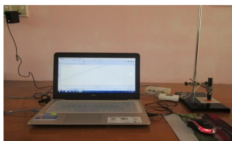
Figure 3. Measurement of gamma radiations by G-M sensor at Department of Physics, University of Research Centre, Monywa
